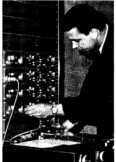
Dr. Robert Hare explains the use of the Grass Polygraph (cost about $7000), sometimes thought of as a lie detector. It is used in the study of psychopaths and in other ways important to psychology research.
