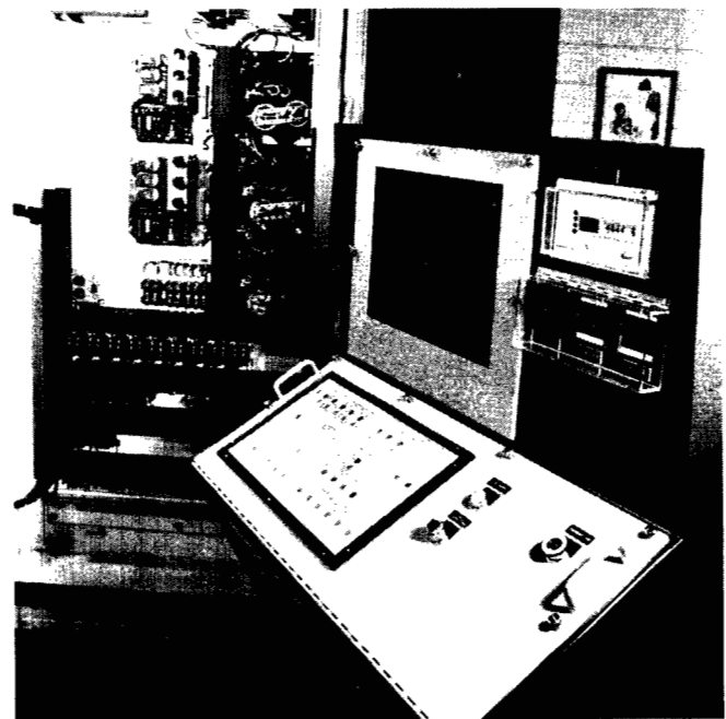
Dynapro Systems Inc., a Vancouver-based Company, developed this machine for industrial program control. The system provides control and monitoring for textile fibre press and baling systems at a South Carolina plant.
