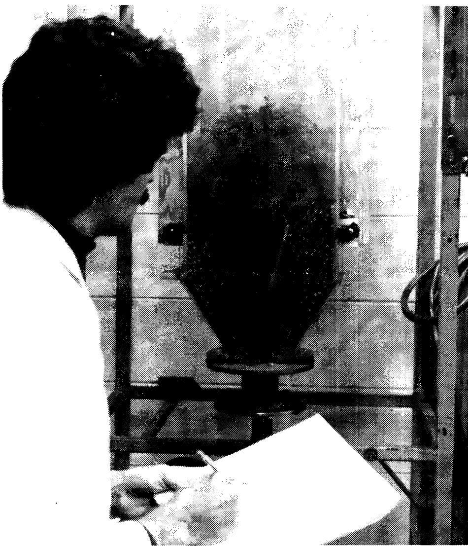
A spouted bed that keeps coal particles in constant motion is used by a research team in UBC's Department of Chemical Engineering. The group has received a $68,000 strategic grant to help try to solve problems in energy production.
