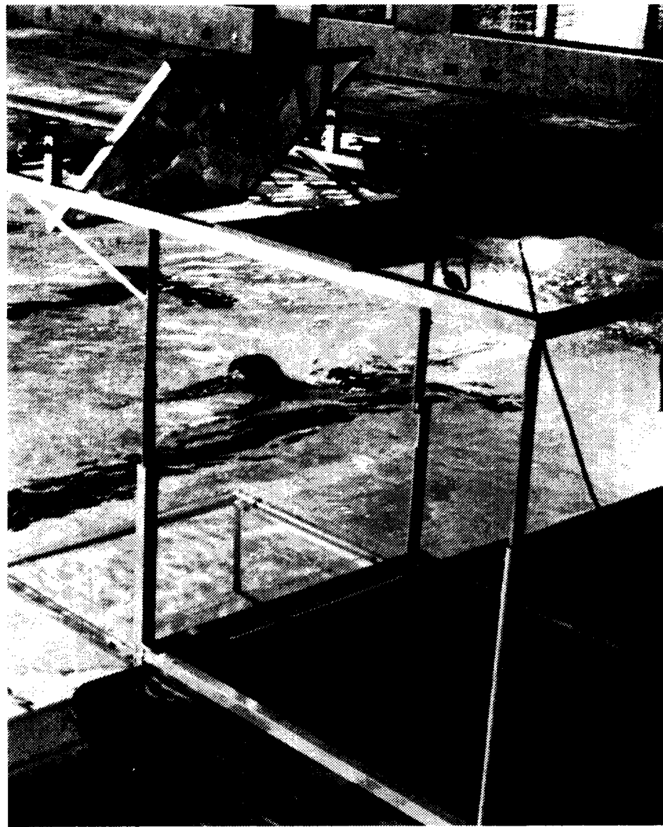
Swimmer is Martin Kai Way of Vancouver Pacific Swim Club, who is participating in UBC Division of Sports Medicine study of knee problems encountered by breaststroke swimmers. Researchers are able to watch and videotape swimmers' technique thanks to ingenious device consisting of two mirrors — one of them underwater — mounted on a metal frame built on UBC campus.
