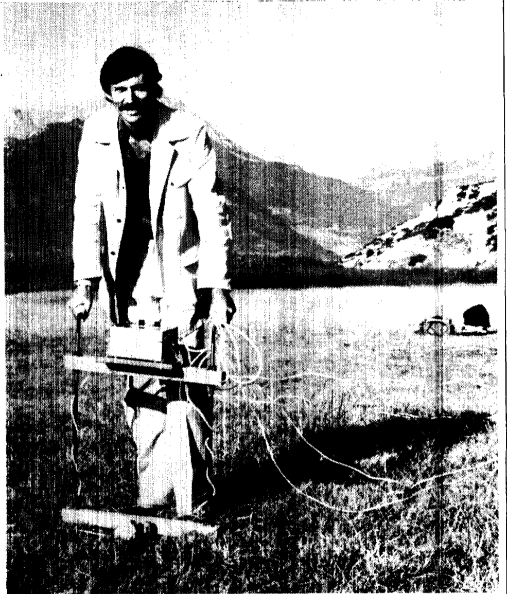
Dr. Hector Williams is the leader of UBC classical archeology team which used geological exploration equipment like this resistivity meter to plot the ruins of buried cities in Greece last summer. See story on Page 2.
