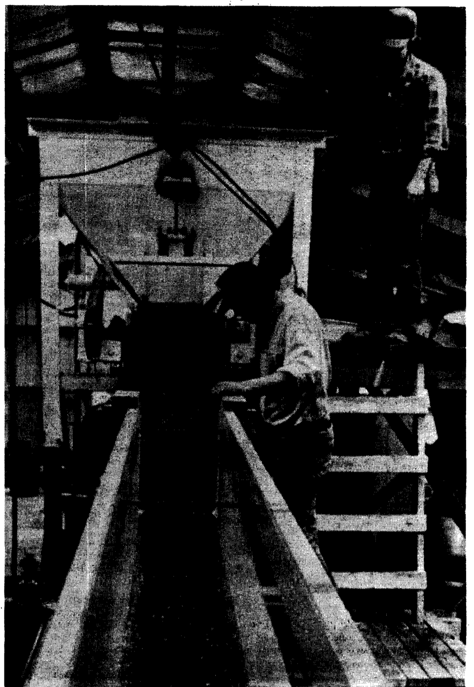
This Yukon sluice box at the Western Canada Hydraulic Laboratories in Coquitlam is being tested for efficiency in recovering placer gold
