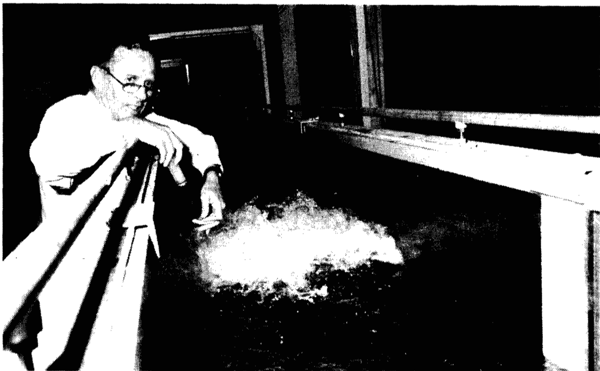
As 6,000 litres of water rush down a 70-foot flume in the engineering lab, simulating the eroding effects of ocean waves, Civil Engineering Professor Michael Quick measures how the water currents move the sediment. The information gathered by Quick's experiments is valuable to marine consultants and others who are trying to protect coastline areas for recreational and marine use.
