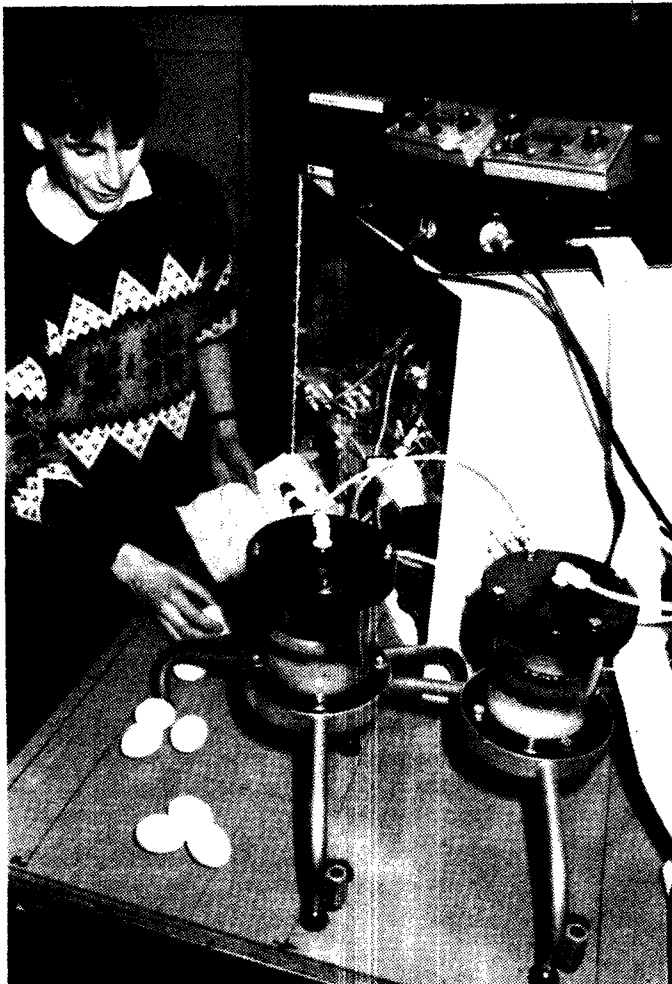
Graduate student Ed Charter shows off an apparatus used to recover an enzyme from egg whites which is used in cheese making. It is on display at the Department of Bio-Resource Engineering.
