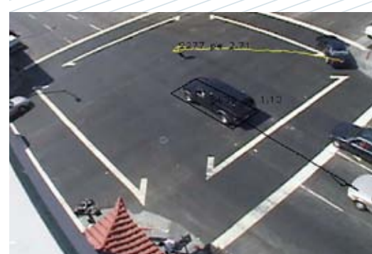
Figure 2 A sample of automatically detected pedestrian-vehicle conflict in a before and after safety study of a pedestrian scramble phase in California.
