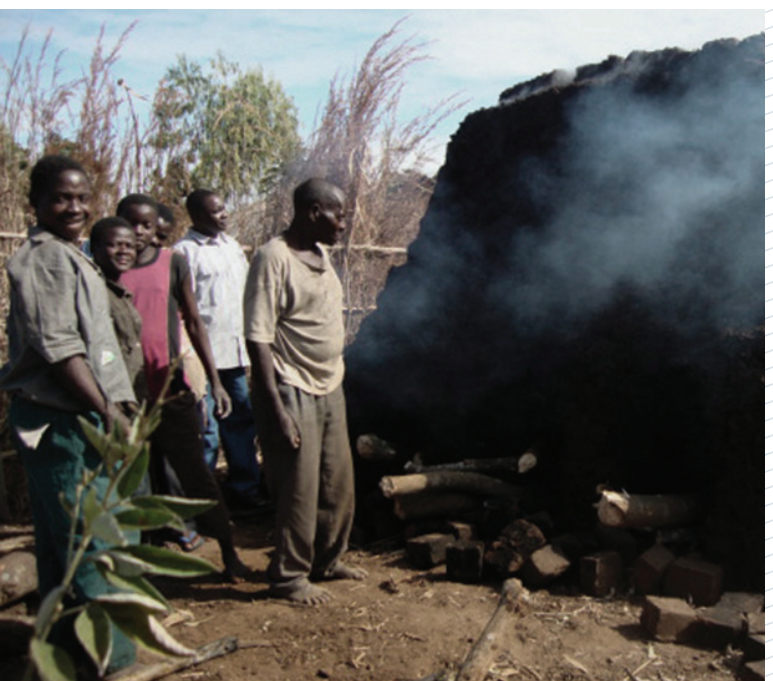
Taken in Chiladzulu in southern Malawi, men are burning bricks in a brick kiln using firewood collected from the surrounding forests.
