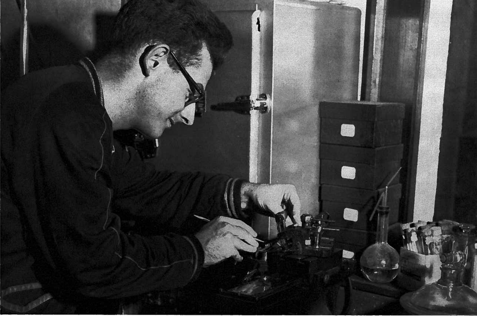
Wood so thin that light can be shone through it is made by Dave Armit, fourth year Forestry student. He is using a microtome, an instrument that cuts sections of wood about 15 microns in thickness for use in microscopic slides. Slides are used for identification purposes in courses on Wood Anatomy.
