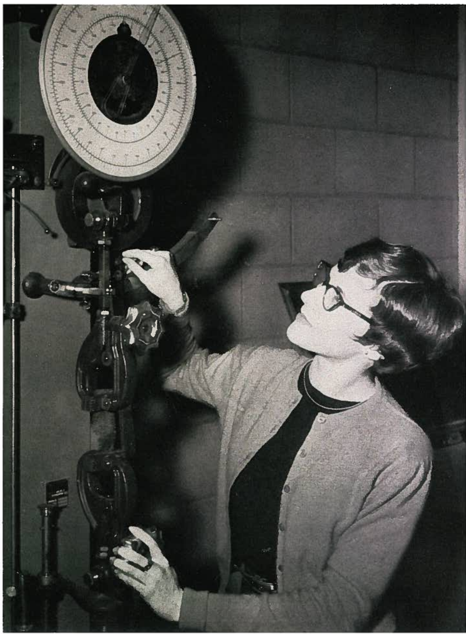
Home Ec apparently involves some engineering, judging by the dials, gears, handles, switches . . . Ruth Cairns take a good look at the robot, a tensile strength machine for testing textiles.
