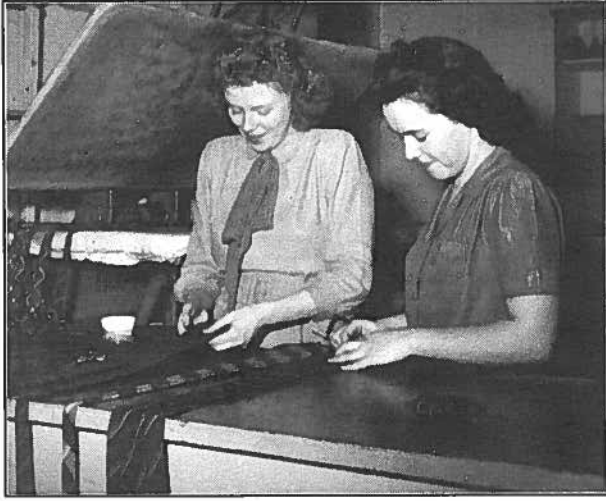
Two Spider Loom workers are shown here inserting a frame inside each tie. Then twelve ties at a time were laid in the big steam press at left rear, for the finishing touch.
