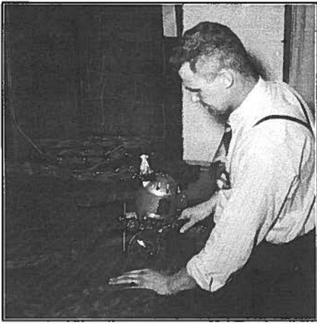
Edgar Bollerup carefully cutting 20 layers of cloth to make ties. The cloth was woven with 31 threads per inch warp and 31 threads per inch weft. The cut must be on the bias (45°) so that the finished tie would not curl. The cutter was new in 1942. Prior to that the cutting was done with scissors - six layers at one time.
