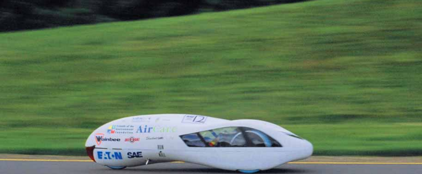
MARK V supermileage vehicle in action. The carbon-fibre car weighs 80 lbs and gets more than 3,000 miles to the gallon.
