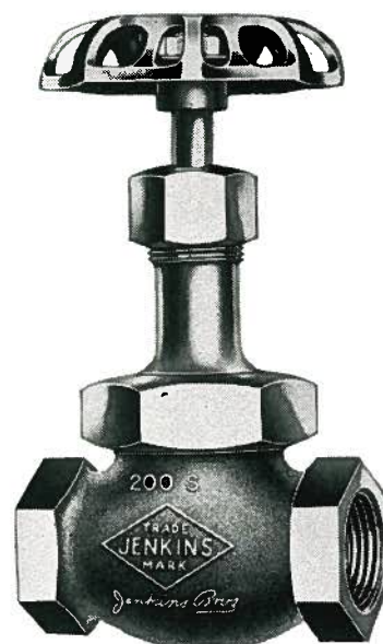
Fig. 2058 Bronze Globe Valve with bevel disc and seat of Wearesist — a special nickel alloy that has greater resistance to wear than that of metals ordinarily used for seating surfaces. These valves can be fitted, if desired, with renewable composition disc or with throttling type disc and seat ring of Wearesist. Suitable for 200 pounds Steam Pressure at 550°F. or 400 pounds Non-Shock Cold Oil, Water, Gas Pressure.
