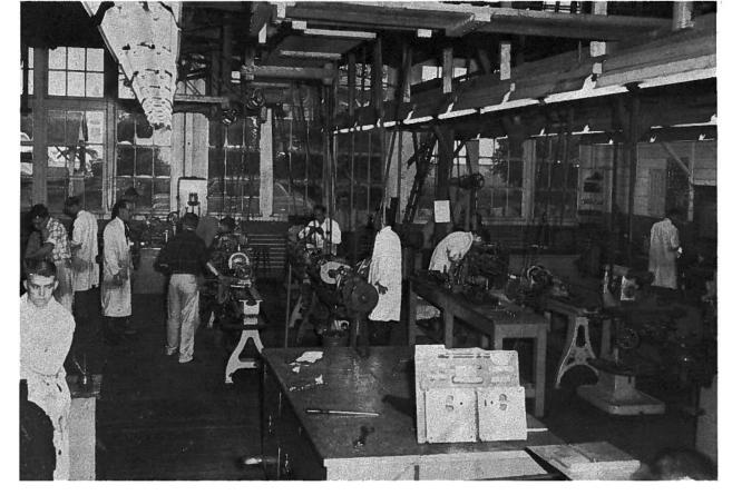
Working on various lathes, milling machines and other assorted mechanical monsters is this class in the Mechanical Engineer's machine shop. Each member of the class is engaged in making an eight-inch bench saw.
